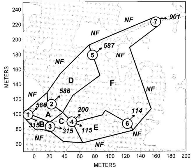
Figure 3. Example treatment zone distribution used in calculating material flux rates within the study area. Example shown is for July 10<sup>th</sup>. Each lettered polygon represents a separate treatment zone. Each numbered circle indicates a water quality sampling location. Shading represents wetted surface area. 'NF' boundaries indicate dry or stagnate areas of no observable flow.
