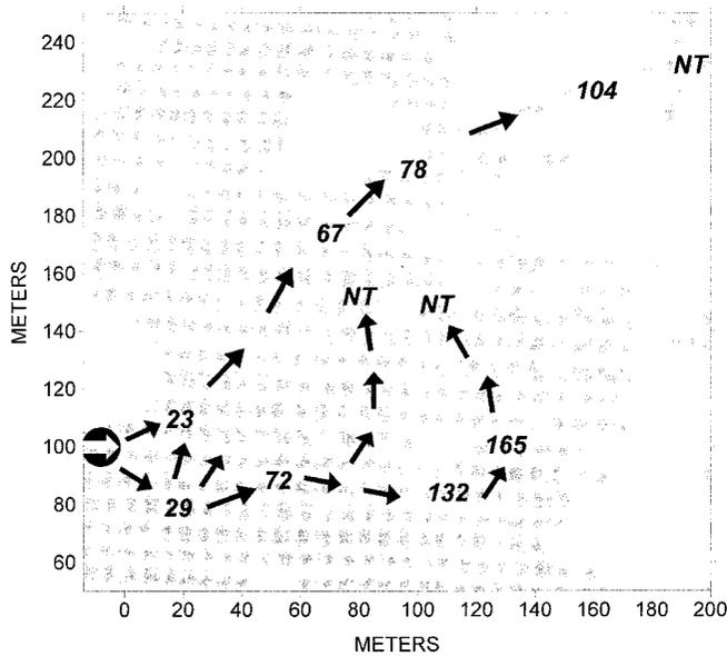
Figure 4. July 10 tracer study results with arrows showing typical primary dye flow paths. Numbers show minimum elapsed travel times in minutes from the pond discharge pipe. Travel times were proportionately shorter or longer for study periods of higher or lower discharge, respectively. 'NT' indicates the location where diffusion, rather than advection, begins to dominate the movement of the leading edge of the dye plume.
