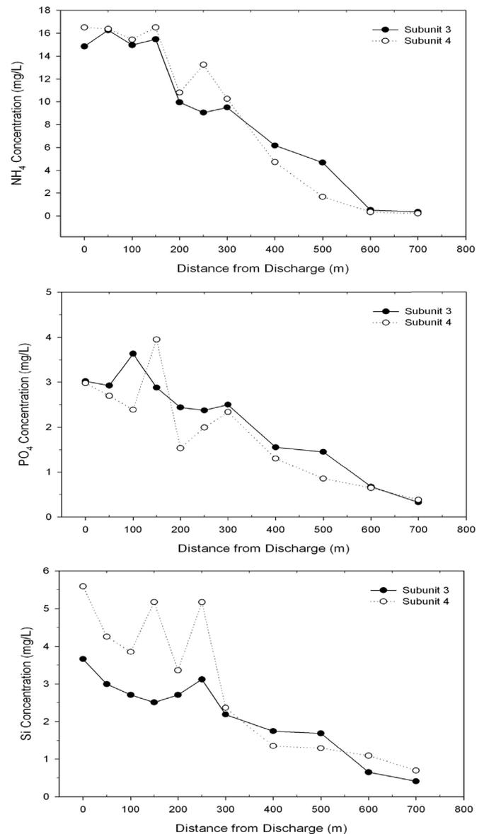
Fig. 5. Surface water quality (NH<sub>4</sub>, PO<sub>4</sub>, and Si) at various distances from the discharge pipe in the Hammond Assimilation Wetland (redrawn from Lundberg, 2008).
