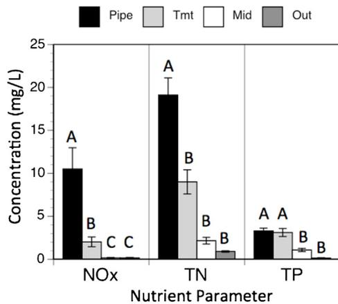
**Fig. 6.** Long-term (2007–2013) water quality data from the Hammond Assimilation Wetland ( $\pm 1$  s.e.). NO<sub>x</sub>: nitrate + nitrite; TN: total nitrogen; TP: total phosphorus. Bars with different letters differ according to Tukey–Kramer multiple comparison.
